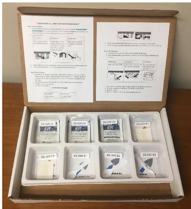
**Fig. 1.** Lead sample collection kit.
